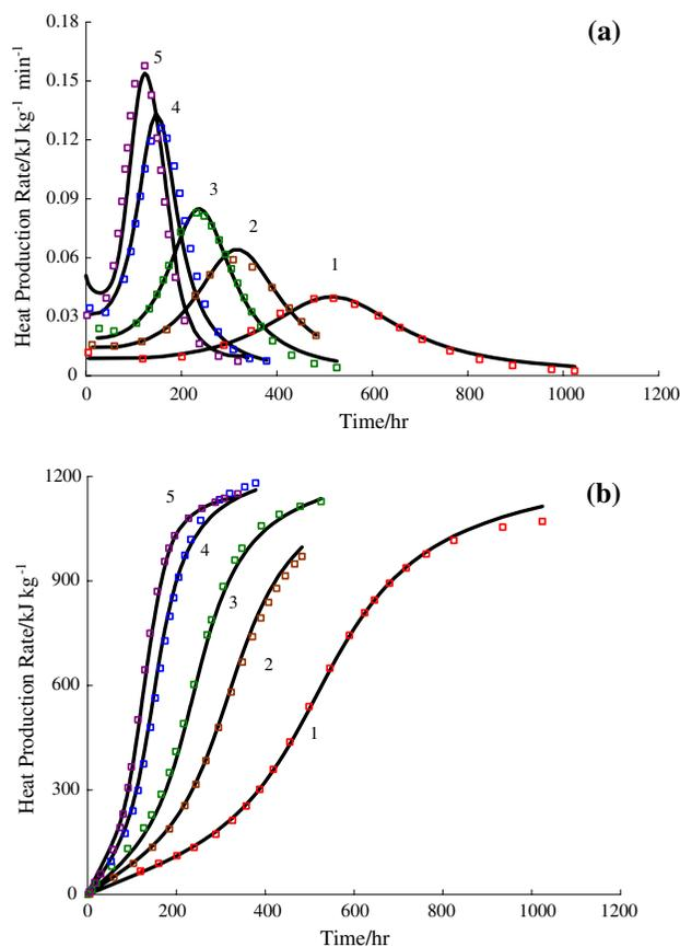
**Fig. 2** Comparison of numerical simulations (—) and experimental data (□□□) at 1—75 °C, 2—80 °C, 3—83 °C, 4—88 °C and 5—90 °C for **a** heat production rate and **b** heat production by the simplified concentration-based model (scheme A)
