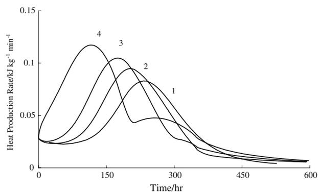
**Fig. 8** Heat production rate v.s. time predictions, assuming various ·OH concentrations in the initial mixture at 83 °C. CHP/cumene/·OH ratio (weight fractions): 1—0.8/0.2/0.0; 2—0.8/0.19/0.01; 3—0.8/0.18/0.02; 4—0.8/0.16/0.04
