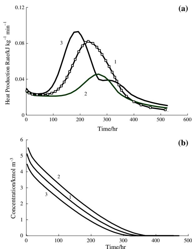
**Fig. 6** Decomposition predictions with various CHP concentrations at 83 °C by scheme B for **a** heat production rate and **b** CHP concentration. CHP/cumene ratio (weight fractions): 1—0.8/0.2; 2—0.9/0.1; 3—0.7/0.3; 4—experimental data ( $\square\square\square$ ) for 80 mass% solution
