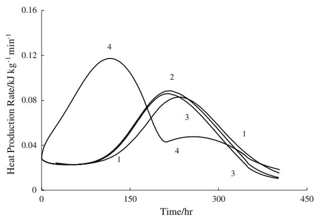
**Fig. 7** Heat production rate v.s. time predictions, assuming elevated concentrations of different radical in the initial mixture at 83 CHP/cumene/radical ratio (weight fractions)—0.8/0.16/0.04: 1—no radicals (CHP/cumene—0.8/0.2); 2— $C_6H_5C(CH_3)_2O$ ; 3— $C_6H_5C(CH_3)_2$ ; 4—OH
