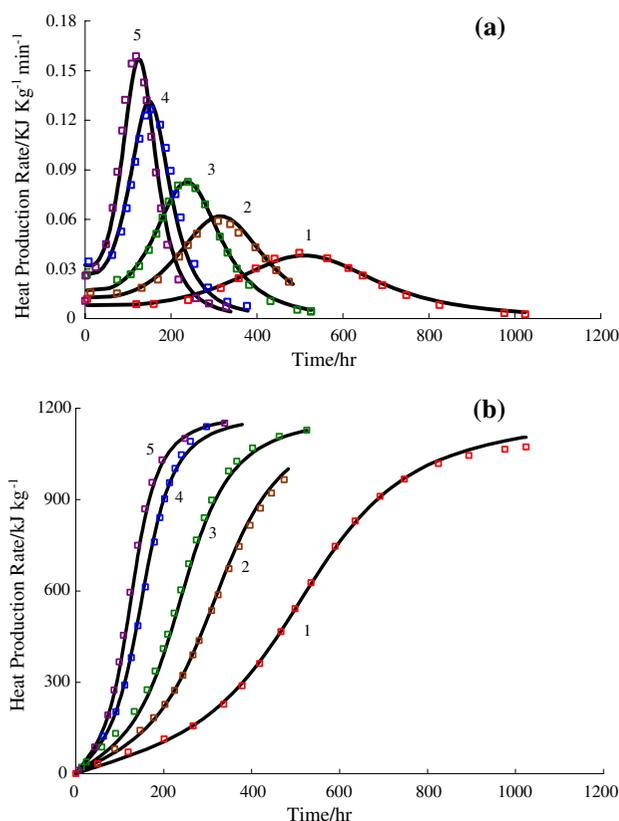
**Fig. 1** Comparison of numerical simulations (—) and experimental data (□□□□) at 1—75 °C, 2—80 °C, 3—83 °C, 4—88 °C and 5—90 °C for **a** heat production rate and **b** heat production by the formal model of full autocatalysis
