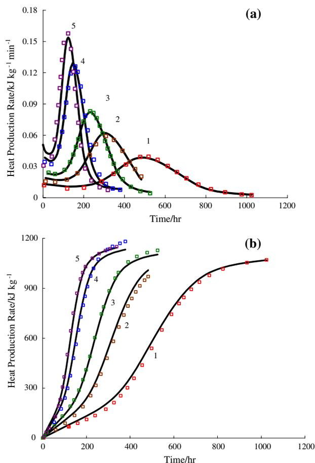
**Fig. 3** Comparison of numerical simulations (—) and experimental data ( $\square\square\square$ ) at 1—75 °C, 2—80 °C, 3—83 °C, 4—88 °C and 5—90 °C for **a** heat production rate and **b** heat production by the meticulous concentration-based model (scheme B)
