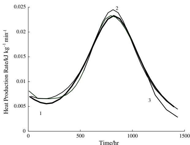
**Fig. 4** Prediction of the decomposition of 80 mass% CHP solution at 70 °C by different models: 1—formal autocatalysis; 2—two-stage scheme A; 3—meticulous scheme B
