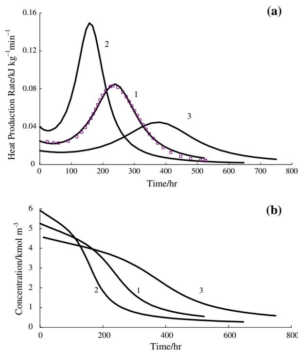
**Fig. 5** Decomposition predictions with various CHP concentrations at 83 °C by scheme A for **a** heat production rate and **b** CHP concentration. CHP/cumene ratio (weight fractions): 1—0.8/0.2; 2—0.9/0.1; 3—0.7/0.3; 4—experimental data ( $\square\square\square$ ) for 80 mass% CHP solution
