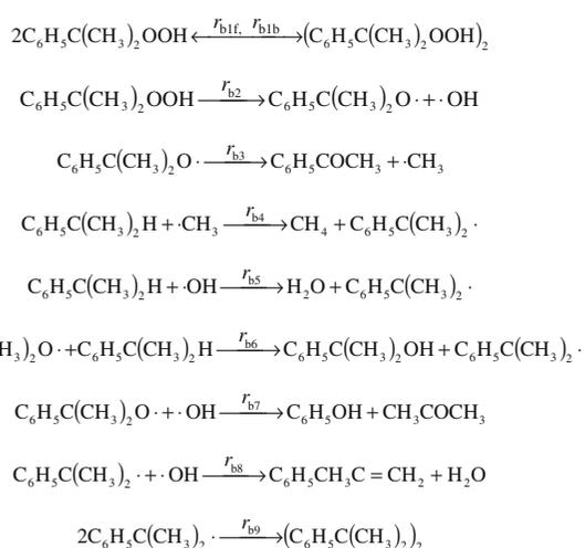
**Scheme 2** The homolytic decomposition scheme (scheme B) of CHP
