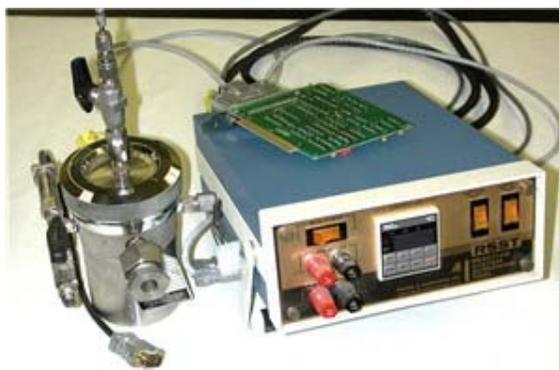
Fig.2.3. RSST including a pressure vessel and control unit
